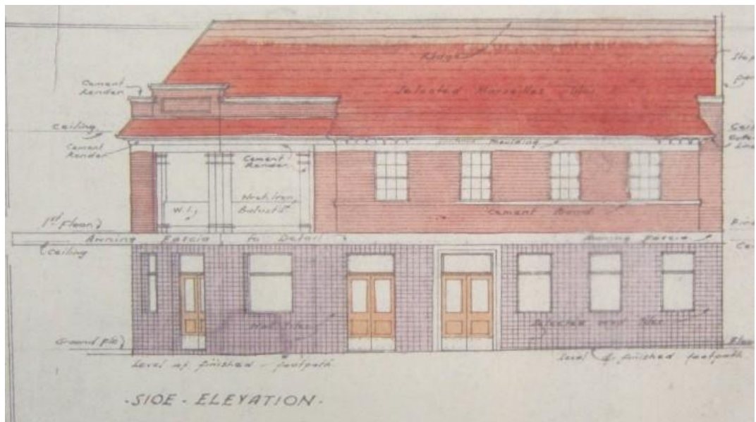
Figure 11 Portion of a drawing prepared in the office of Rudder & Grout during the first half of 1934 describing the Garden Street facade of the new Alexandria Hotel. Source: State Records AO Plan 69570.
